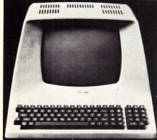
Upper case and lower case; 15 baud rates: 75 to 19,000 baud; dual intensity; 24 x 80-char. display, 12 x 10 resolution. Numeric pad. Programmable reversible video; aux. port; self-test mode; protect mode; block mode; tabbing; addressable cursor. Microprocessor controlled; programmable underline; line and character insert/delete.
